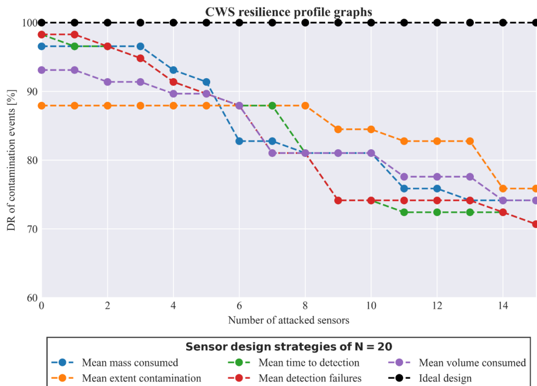
Figure 8. Resilience profile graphs for the five objective functions used to generate topologies of 20 sensors.
