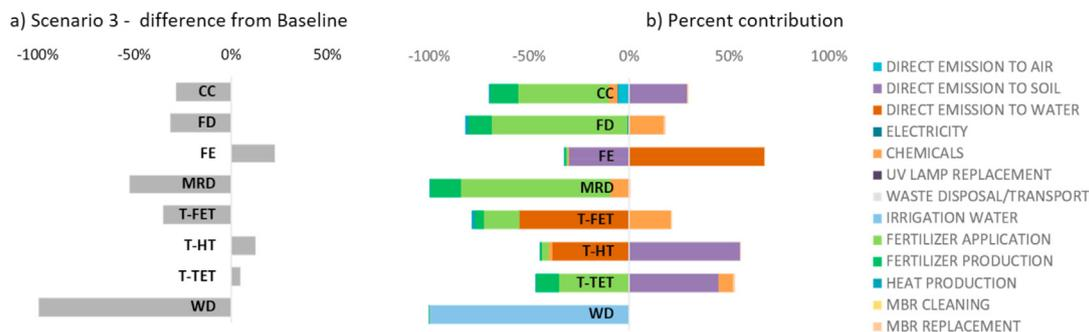
Fig. 7. Environmental performance of UASB followed by AnMBR relative to baseline scenario: a) as overall relative differences in each category; b) percentage contribution analysis based on the individual processes and sources of impact.
