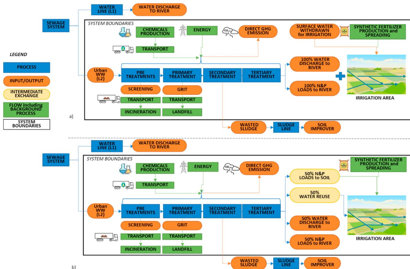
Fig. 2. System boundaries for the life cycle assessment: a) baseline configuration; b) alternative scenarios.
